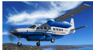
ZA600: Adapted Technology 100 – 750 kW LTPEM Fuel Cells (~85°C) • Superstack Concept • Central Compressor • In-House E-Motor + Inverter • High Power Density System
